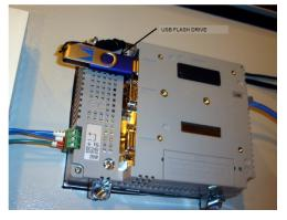
The saved files on the USB flash drive can be accessed by any PC with a USB drive port.
