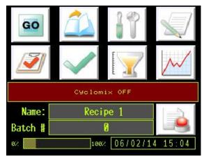
The Batch *#* is a user defined field which the operator can use to track production data. The parameter is numeric only. The batch *#* is saved with the consumption data.
