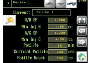
recipe by using the increment and decrement arrow keys. Once the operator has found the recipe the operator
