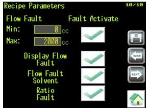
The end user can enable or disable the "Solvent Flow Fault" by selecting its icon.
